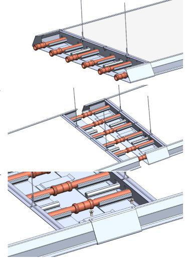
Slide the cover strip back to hide the exposed connections and secure with self-tapping screws.
