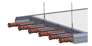
Slide the cover strip over the first radiant panel.
