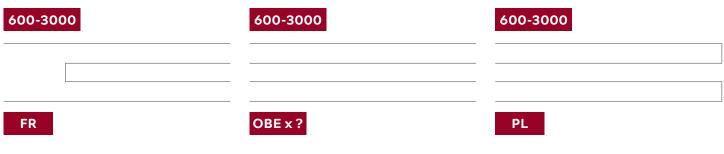
When joining panels longer than 3000mm, a FR & EP panel will complete the panel assembly. The OBE panel can be used to lengthen the complete panel to the desired length.
